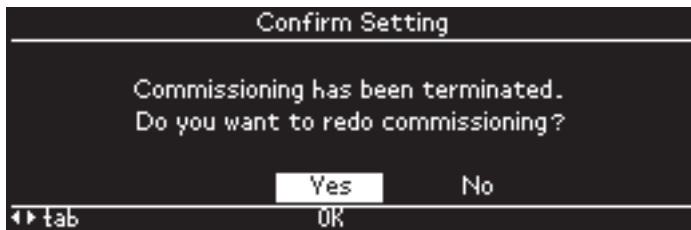
Fig. 77. Failed commissioning step
