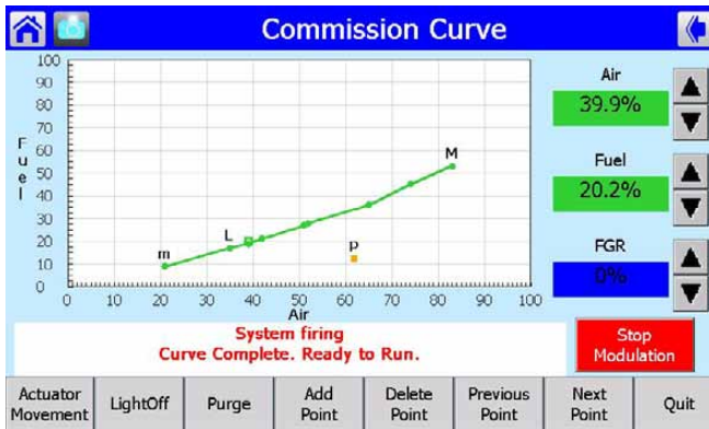
Fig. 60. Completed Commissioning Curve.
